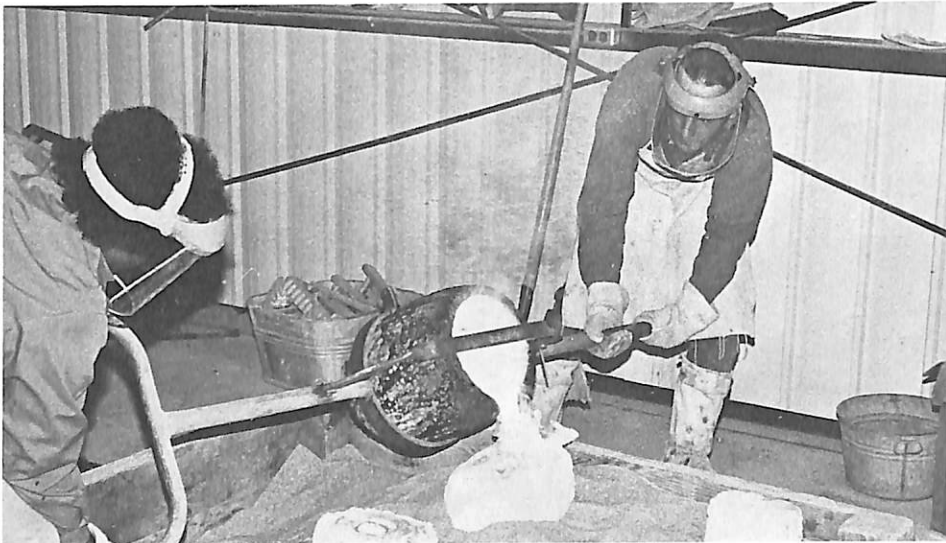
Yes, this is a campus photo. Dana is one of only a few colleges in the area with a sculpture foundry. Here students Reginald Tullos '82 (left) and Mark Jorgensen '80 pour molten bronze from the crucible into molds buried in sand.
