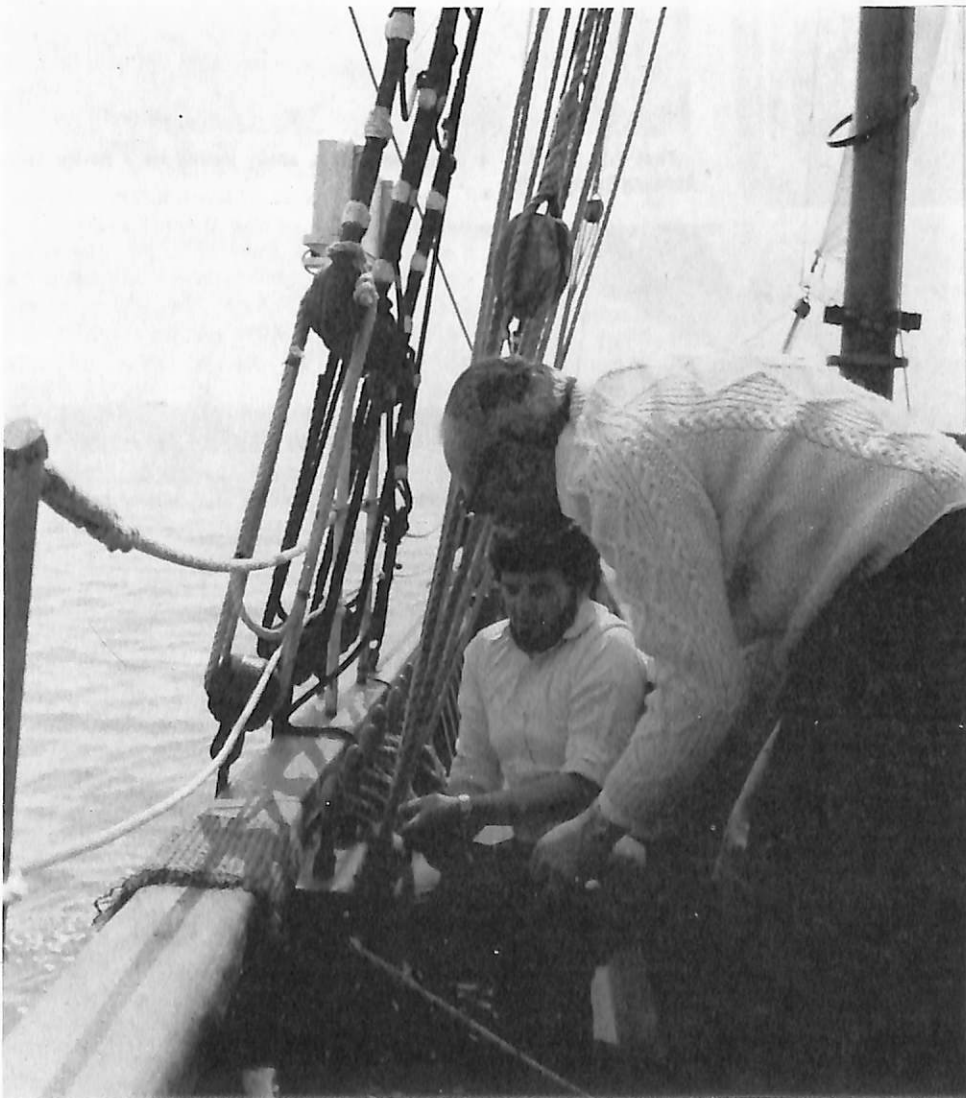
Part of the crew investigates how part of the rigging works — how to wrap a line around a belaying pin.
